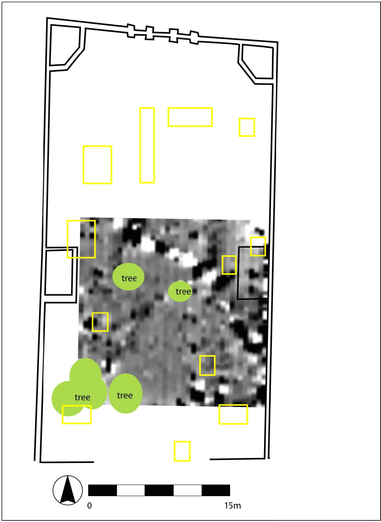
Figure 9. Results of the magnetic gradiometer survey of the Aiken-Rhett house back lot.
